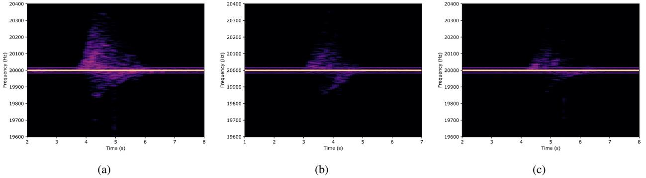
Fig. 3: FFT spectrograms of open events of Door2 when the smartphone was placed (a) 1 m away from the Door2 (b) 3 m away from the Door2 (c) 5 m away from the Door2.
