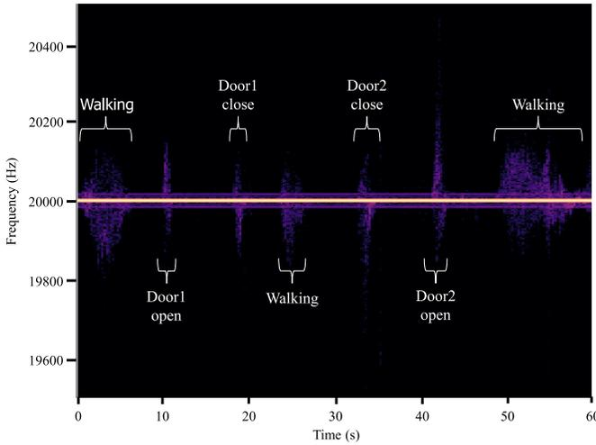
Fig. 4: FFT spectrogram of one data set (front channel) where the smartphone was placed 2.7 m away from the Door1 and 3.6 m away from the Door2.
