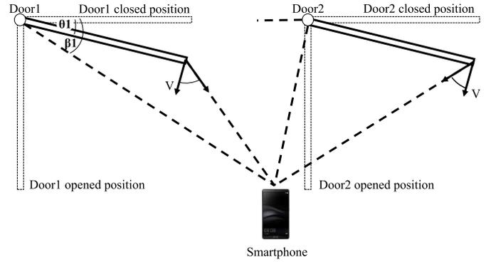
Fig. 1: Relationship between the location of the smartphone and the shape of the frequency distortion expected.
